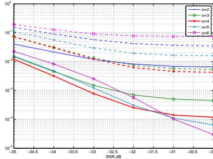
Figure 2: Dependencies of  $P_e$  (probability of erroneous decoding, shown with solid lines) and  $P_d$  (denial probability, shown with dashed lines) on the SNR value in dB (for rate 1/4 inner code and  $K=200$ )
