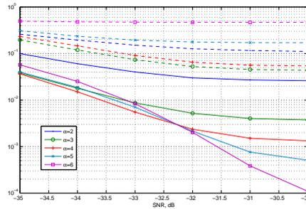
Figure 1: Dependencies of  $P_e$  (probability of erroneous decoding, shown with solid lines) and  $P_d$  (denial probability, shown with dashed lines) on the SNR value in dB (for rate 1/3 inner code and  $K=200$ )
