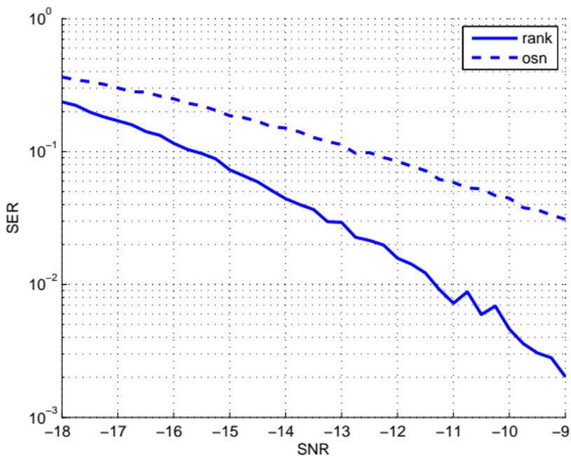
Рис.: Collisions in 15% of user area with interference power 30db
