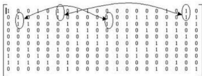
Cycles of the length 4 in the parity check matrix of the (3, 10) LDPC code
