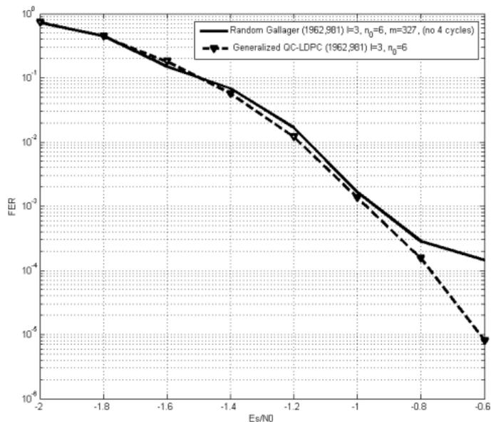
The dependence between the error probability per frame (FER) and the signal-to-noise ratio ( $E_s/N_0$ ) for the random Gallager code and code from  $\mathcal{E}_{QCC}(l, n_0, m)$ .
