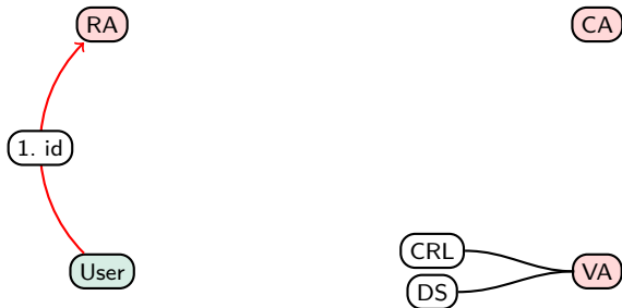
FIGURE: The enrollment/rekeying phase of a PKI
