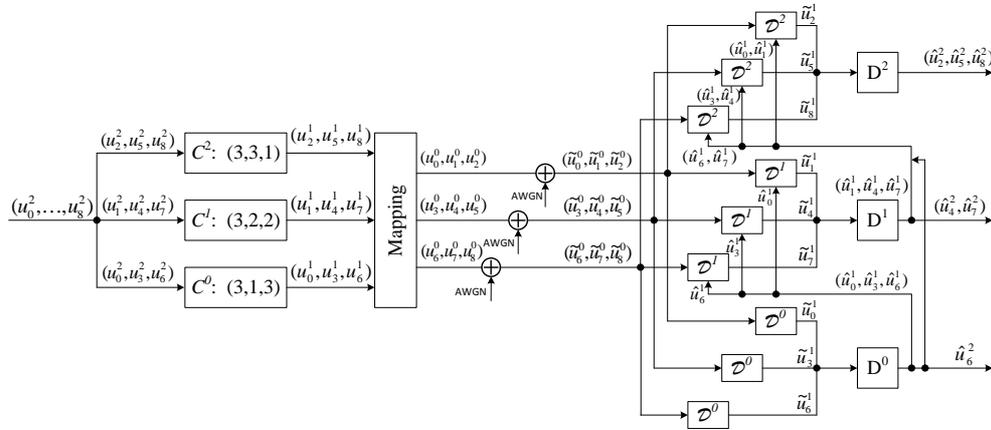
Figure 2: (9, 6) polar code as a multilevel code
