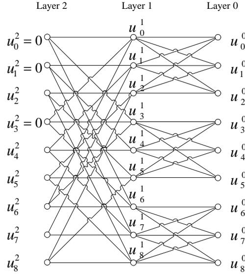
Figure 1: Encoding scheme for (9, 6) polar code
