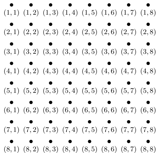
Figure 1: Indexing a 64-QAM constellation
