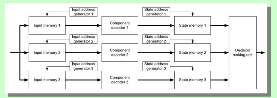
A simple sequential approach can be employed to decode this code in hardware (either FPGA or ASIC). Each component code decoder processes one bit per cycle.
