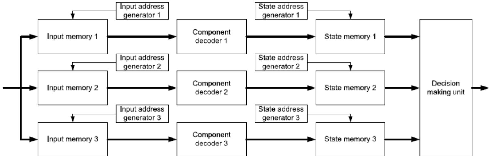
A simple sequential approach can be employed to decode this code in hardware (either FPGA or ASIC).
