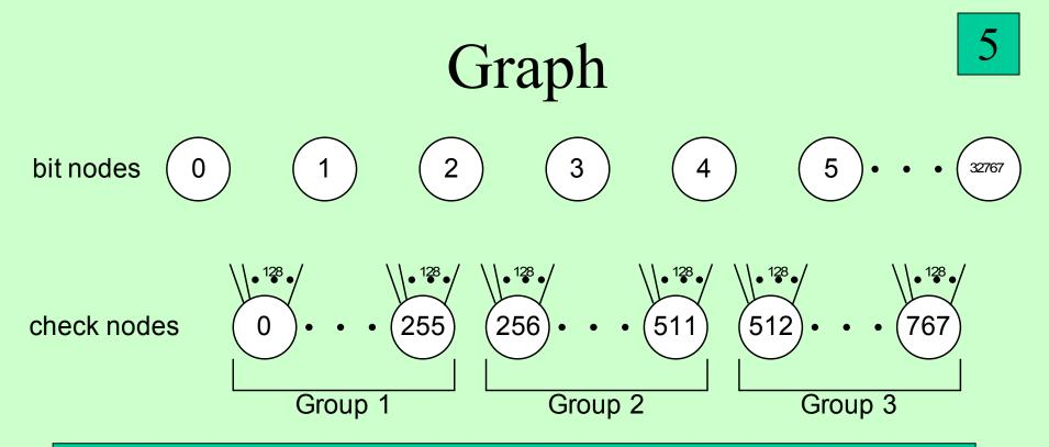
The check nodes are divided into three groups. Each check node represents an extended Hamming codeword.
