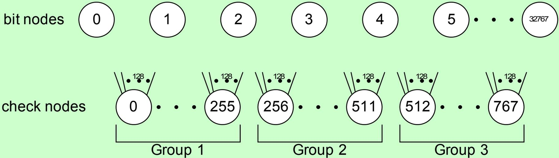
The check nodes are divided into three groups. Each check node represents an extended Hamming codeword.
